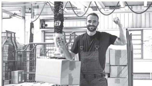
Thanks to the new two-button operation, the specialists control the up and down movement intuitively
